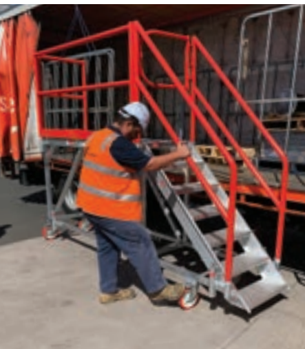
Place in position & lock castors
