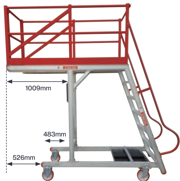
Clearance for Cantilever Platforms
